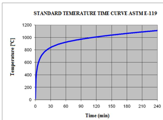
*Figure 2. Standard Temperature-Time Curve ASTM E-119 [4]*
