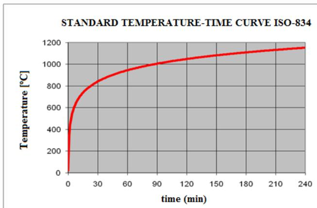
Figure 1. Standard Temperature-Time Curve ISO-834 [4]
