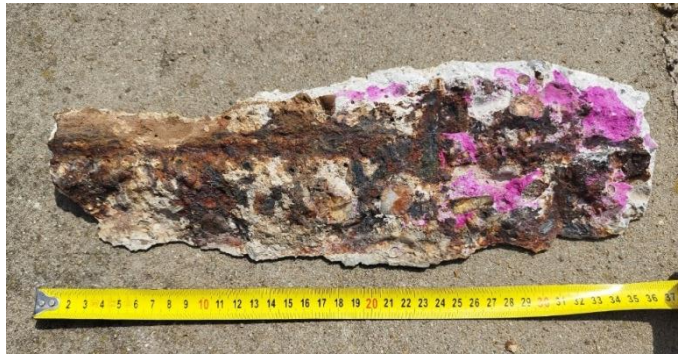
Figure 5: Due to the porosity of the concrete and the looseness of the concrete cover, carbonation is significant, and the concrete is rusty in several places
