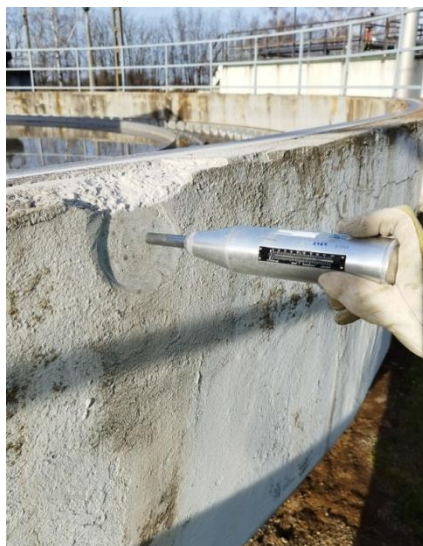
Figure 4: Concrete strength measurement on the tank edge
