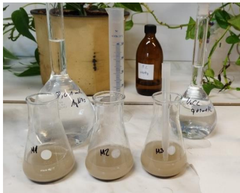
Figure 6: The measured drill dust sample homogenized with distilled water
