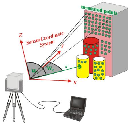
Figure 1: The principle of tachymetric Laser Scanning [11]
