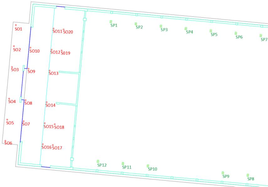
Figure 5: Identification of circular (red) and rectangular (green) columns from the object's top view
