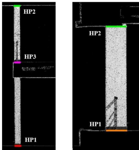
Figure 6: Positions of cross-sections on a circular (left) and rectangular (right) column
