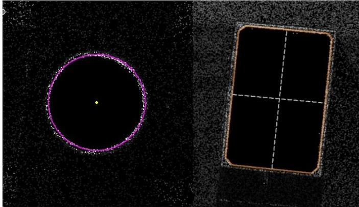
Figure 7: Extraction of cross-sections of columns from the point cloud
