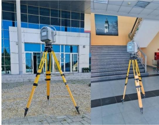
Figure 2: *The Trimble TX-8 scanner in front of the entrance to the sports hall (left) and during the scanning of the interior of the hall (right)*
